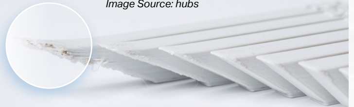
The effect of increasing overhang angle (in increments of 5°) on print quality. The maximum angle shown is 70°.
