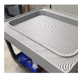
This innovation allowed for rapid and costeffective production of thermoforming molds, circumventing the need for a new tool maker.
