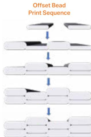
With conventional slicing techniques the weakest portion of the part is the X/Y plane.
